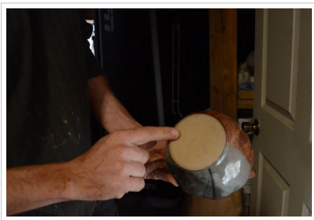
Ferguson shows the speckling pattern that appears in pottery when manganese is mixed into the clay.
